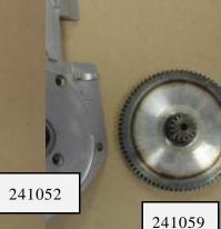
Far left, pry large gear (241059) with small sprocket attached off cover plate.
