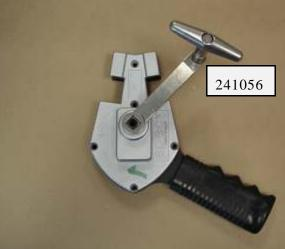
At left, handle attached to pistol housing with cover plate screws (501035) and nuts (506017).
